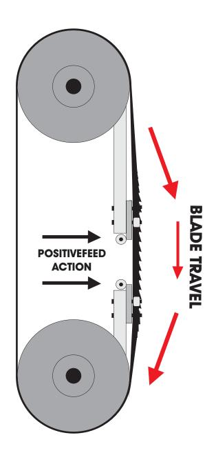
**"POSITIVE FEED"** Action (exclusive to all MetalSawz Models) preloads the saw blade to increase tension between the blade guides by up to 15% This produces cutting rates approximately 15% faster than conventional saws with no appreciable loss of blade life. This feature also eliminates the need for expensive "Positive Rake" or "Hook Tooth" saw blades.
